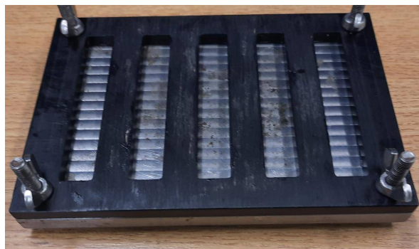
Figure 5. The mould for five samples, each 90mm x 14mm x 7mm.
