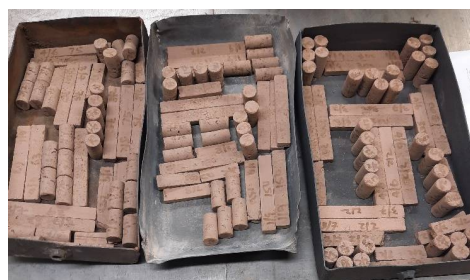
Figure 7. Rectangular and cylindrical samples arranged and ready for firing
