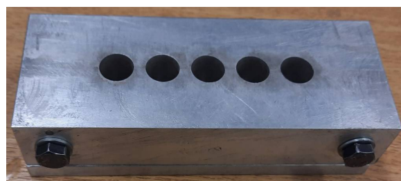
Figure 6. The mould for cylindrical samples for compression tests
