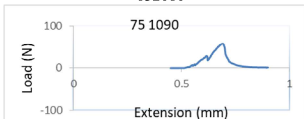
Figure 10. The load-extension curves of sample 751090
